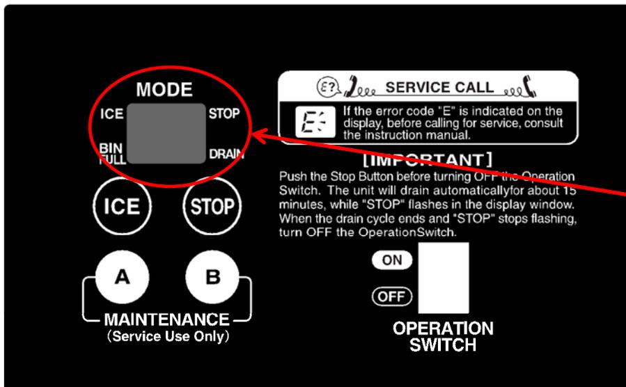
When an error occurs, "E\_" or "c\_" will appear in the display. Some of the "c\_" errors are not displayed and must be checked by the error log.
